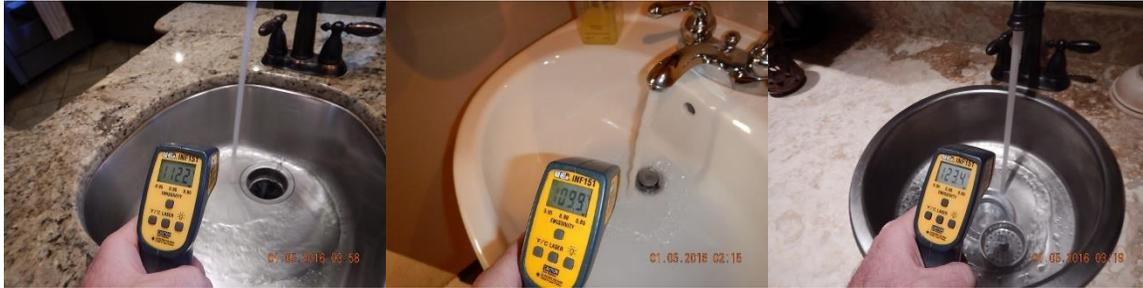
Infrared Thermometer was used throughout the house to verify hot water at the Kitchen and Bathrooms, Laundry Room, and Bar areas during the Home Inspection
