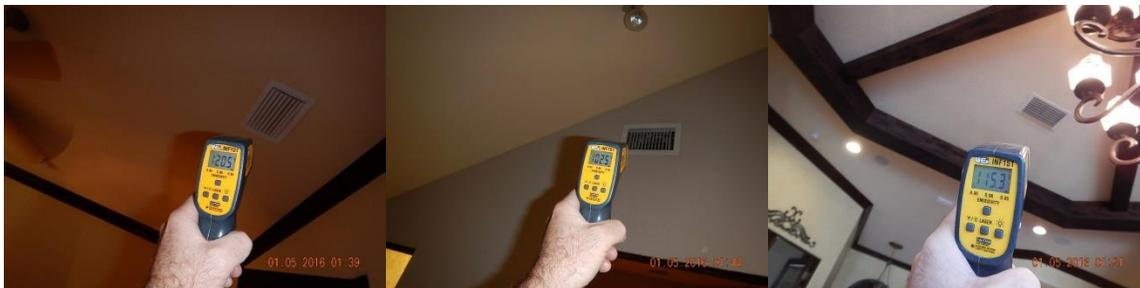
Infrared Thermometer was used to confirm the systems produced heat when operated during the Home Inspection
